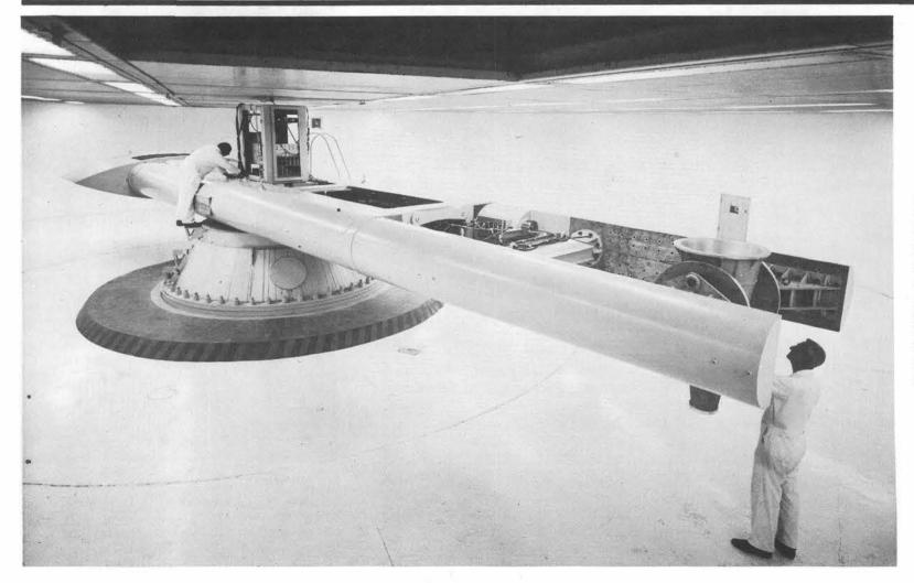
IT GOES ROUND & ROUND — Sandia's centrifuge, located in Area III, was designed to test nuclear weapon hardware (which it still does) and has now been found useful in scale model testing of geologic phenomena such as earth subsidence over coal mines. See article on page four.
